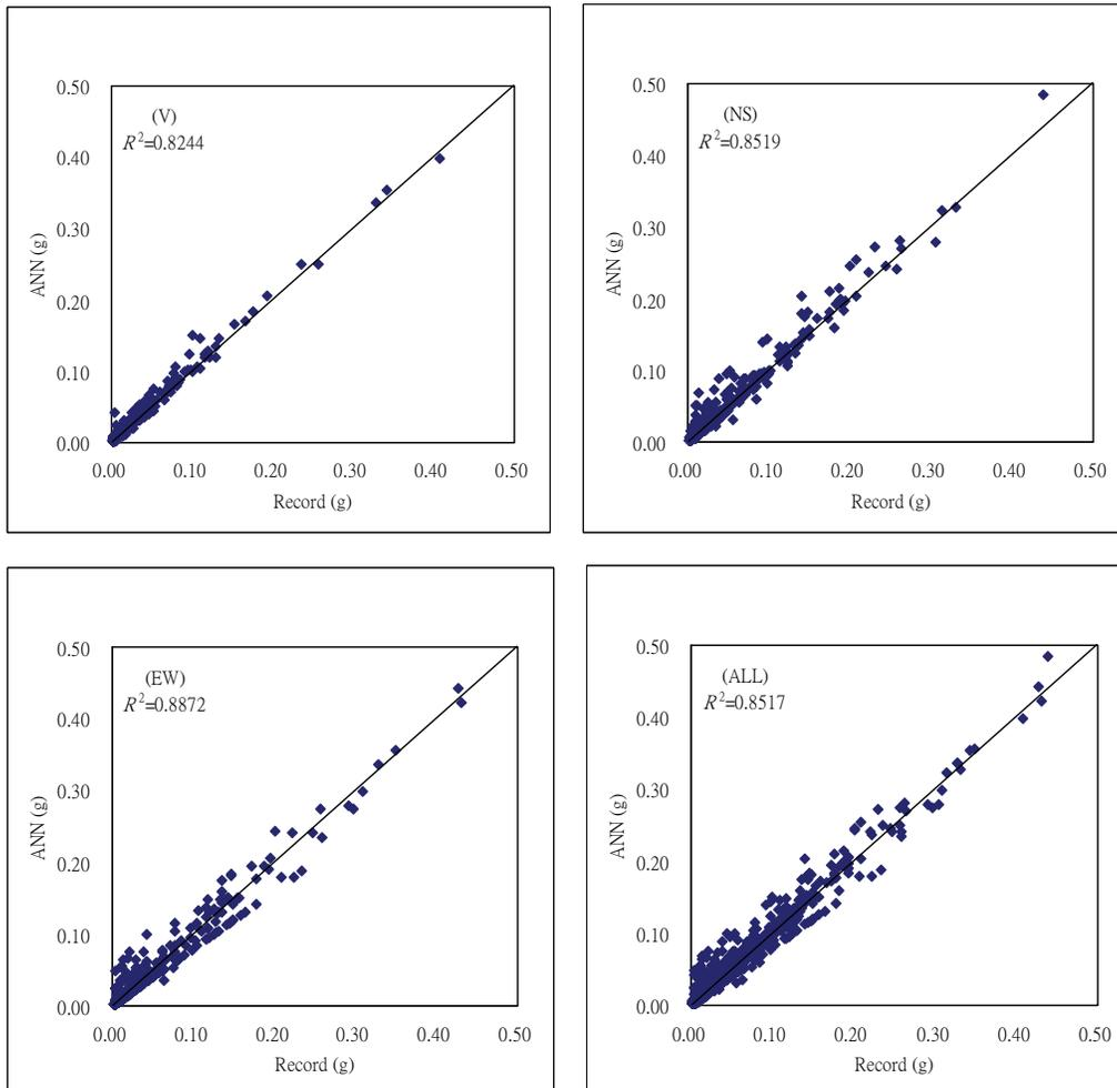
Figure 6: Comparison of neural network model estimations and records, (a) V direction, (b) NS direction, (c) EW direction, and (d) three combined directions.
