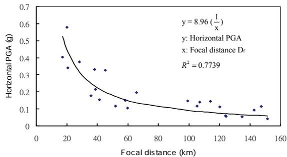
Figure 11: The curve fitting model between horizontal PGA and focal distance.
