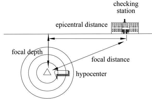
Figure 4: Definitions of parameters for a typical earthquake wave propagation.
