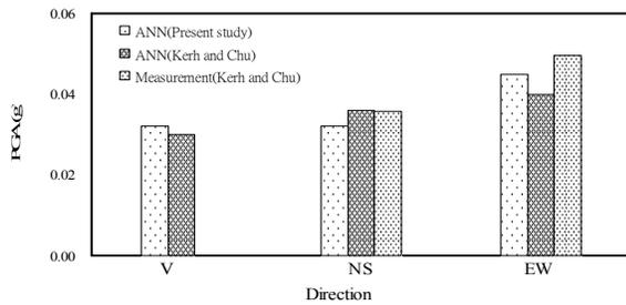
Figure 7: Comparison of ANN estimated PGAs with microtremor measurements (B05).
