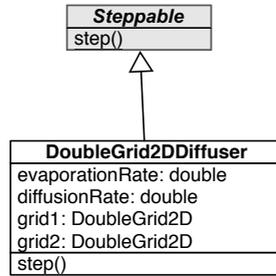
FIGURE 13.4 UML diagram of the `Double2DDiffuser` class.
