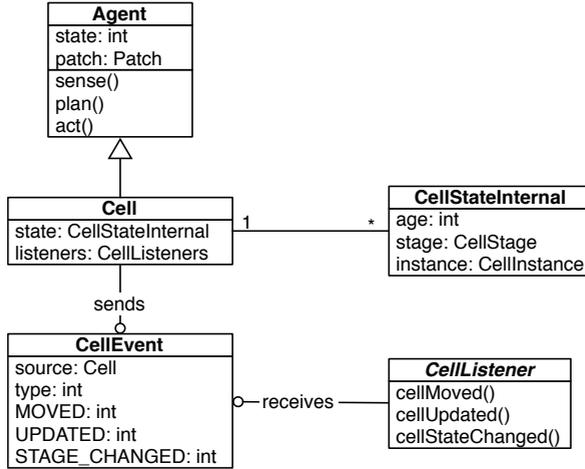
FIGURE 13.6 UML diagram of the Cell class.
